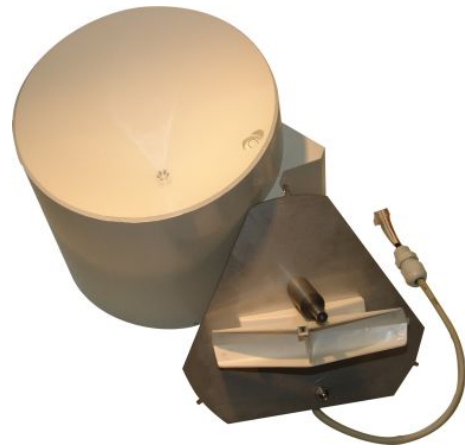
Picture 12: Rain gauge
