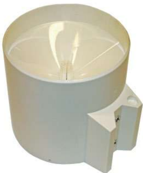
Picture 33: Rain gauge
