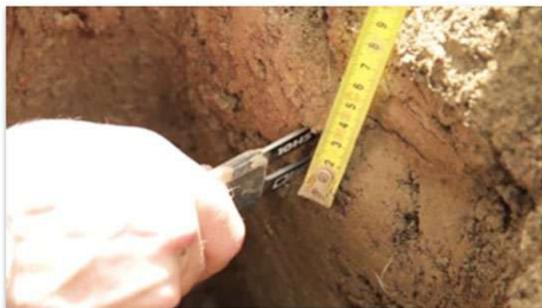
Picture 20: Installing Meter 10HS sensor.
