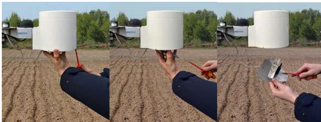
Picture 32: Three steps to open the rain gauge.
