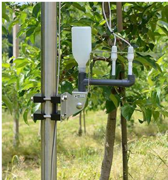
Picture 19: Wet and Dry Bulb Temperature Sensor
