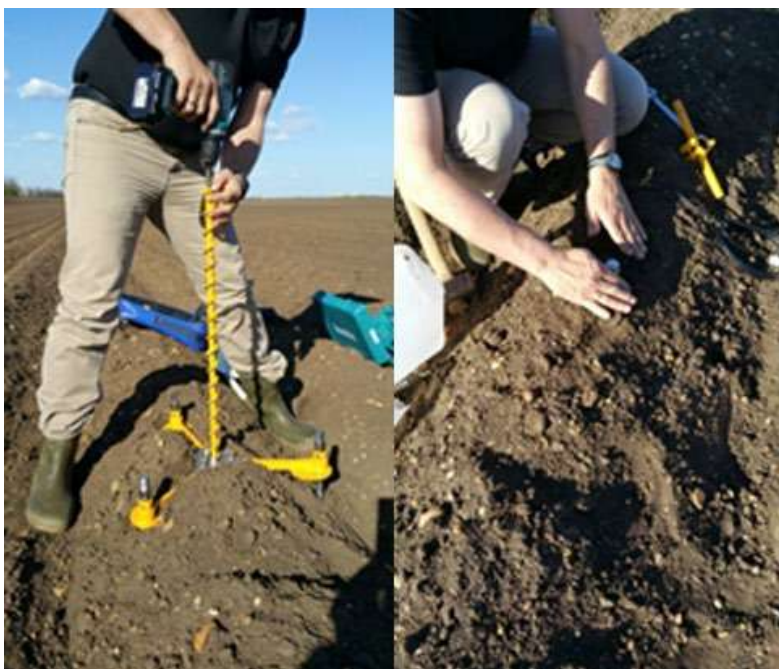
Picture 23: Installation of Drill&Drop probes.
